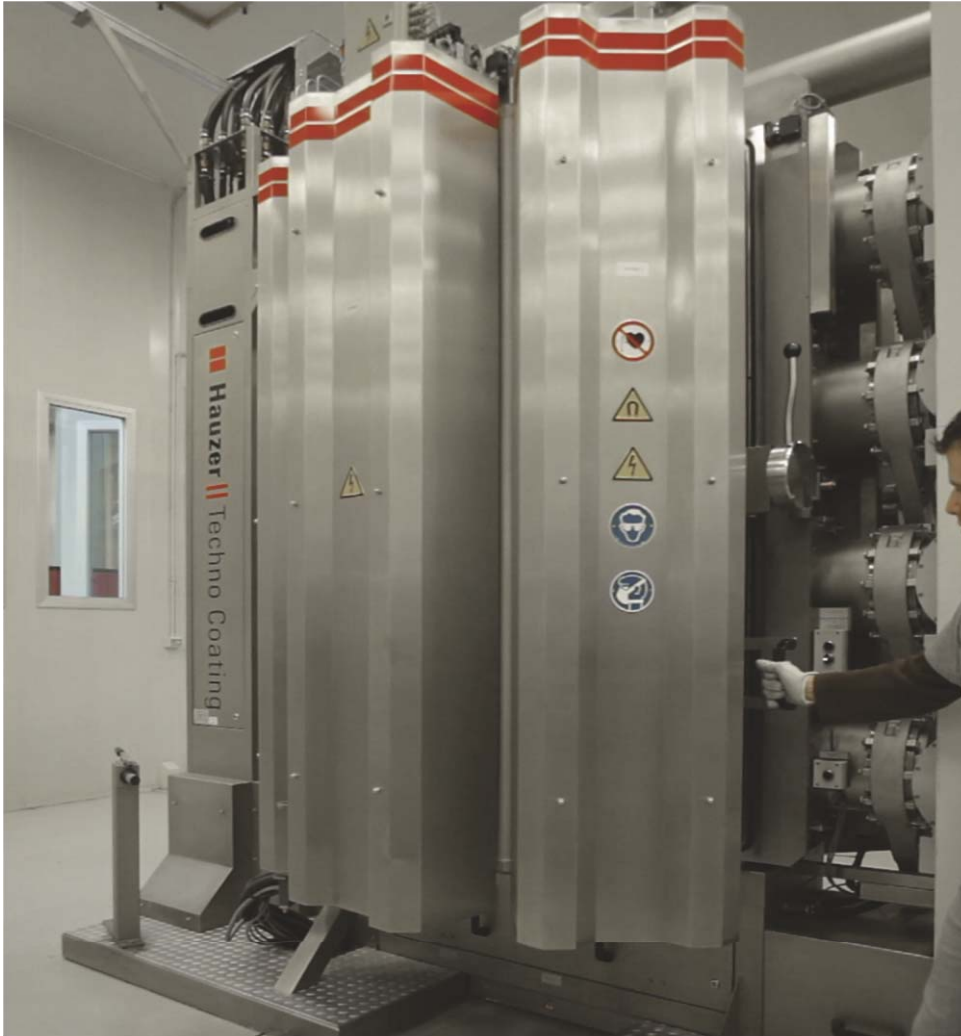
Macchina PVD by Hauzer PVD machine by Hauzer
